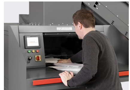
EMERGENCY STOP bar
